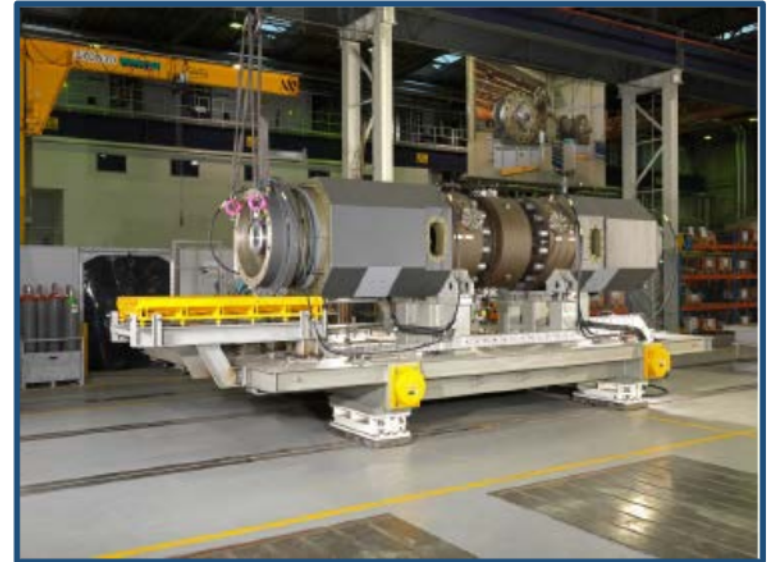
MAN HS electric motor driven tandem unit
